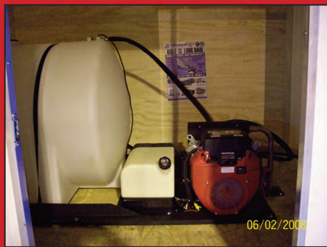
11.5 gpm, 2500 PSI, 325 gallon water tank and hot water option mounted in a customer's enclosed trailer.
