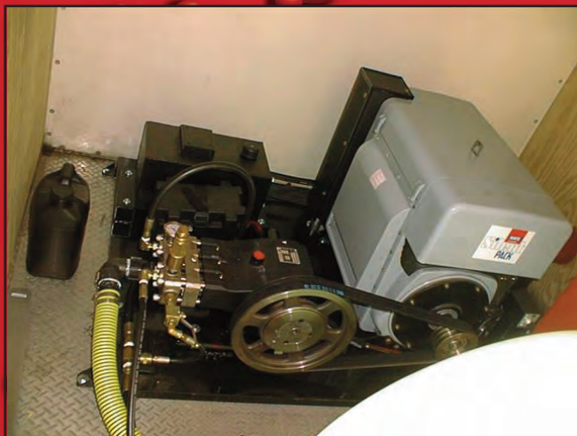
18 gpm, 4000 psi, Hatz Quiet Pack skid.
