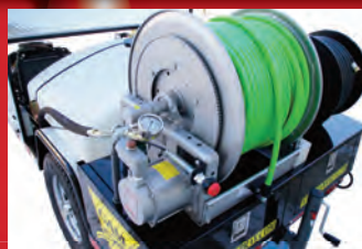
Rear mounted controls include a pressure gauge, water shut-off, remote throttle control,
