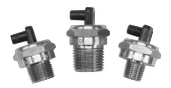
Protects the pump from damaging heat build-up while it is in bypass mode. The thermal relief valve, sensing a rise in temperature, opens and discharges a small amount of heated fluid. This allows cooler water to enter the system and cool the pump. When the gun is discharged the cooler water will cause the valve to close immediately.
